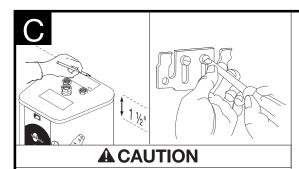
Property Damage: Do not connect the electrical power until the tank is full of water. Failure to comply will burn out the heating elements.
