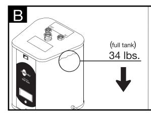
☐ Ensure wall or cabinet is strong enough to hold the weight of a full heater. The model W152 tank holds 2-1/2 gallons and weights 34 lbs. when full.
