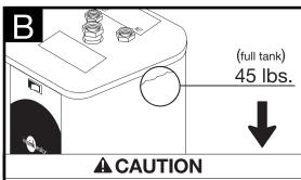
Property Damage: Do not connect the electrical power until the tank is full of water. Failure to comply will burn out the heating element.
