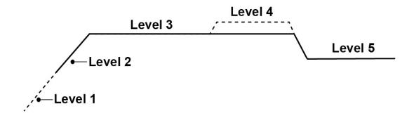
**Soft Charge**- When batteries suffer an over-discharge, the controller will softly ramps the battery voltage up to 10V.
